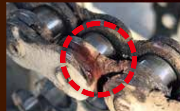
seal ring's deterioration, pin/bushing wear, steel powder oxidizing
