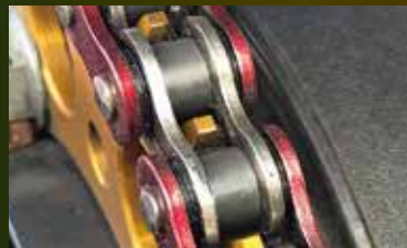
well-lubricated and in good condition
