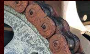
seal ring's deterioration, pin/bushing wear, steel powder oxidizing
