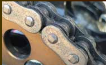
rust on pin/plate surface
