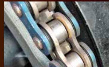
dry surface, lack of lubrication
